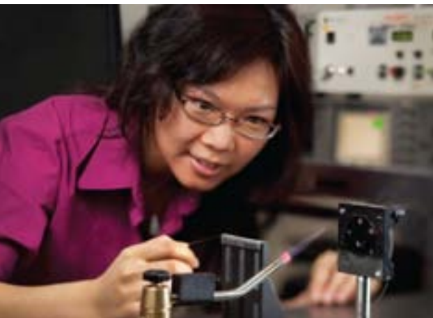
Dr. Xingwei Wang heats an optical fiber taper in her lab at UMass Lowell. She received a 2008 New Investigator Grant from the Massachusetts Life Sciences Center to support her efforts to create a miniature label-free biosensing probe for the rapid detection of viruses, bacteria, and cells.
